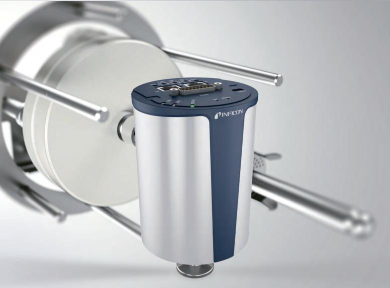
INFICON Stripe high-speed Capacitance Diaphragm Gauges are the fastest, highly accurate vacuum measurement instruments available. With a less than 1 ms response time combined with the EtherCAT fieldbus interface it opens up a total new field of applications. The proven temperature controlled, corrosion resistant, ultra-pure ceramic sensor provides superior span stability over many years paired with state-of-the-art zero stability.
