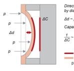
Direct pressure measurement bv diaphragm ∆d ~ p Capacitance readout  $\frac{1}{\Lambda C} \sim p$ Electrode Diaphragm p = pressure
