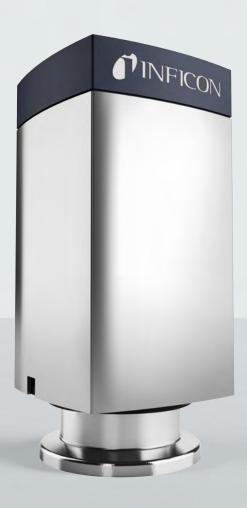
The INFICON Gemini Inverted Magnetron Vacuum Gauge is the workhorse for all vacuum measurement application. Gemini combines two sensor systems into one small device to measures from atmosphere to 1x10-9 mbar. The patented (pending) ultra-low magnetic stray field design opens up a whole new range of applications. A unique interchangeable dual chamber sensor unit avoids cleaning cycles and reduces maintenance, making Gemini the most robust and economical vacuum gauge of its kind.
